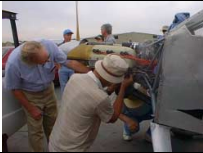
Dennis Cullum assists Paul Hanson in the reinstallation of his Jabiru engine.
