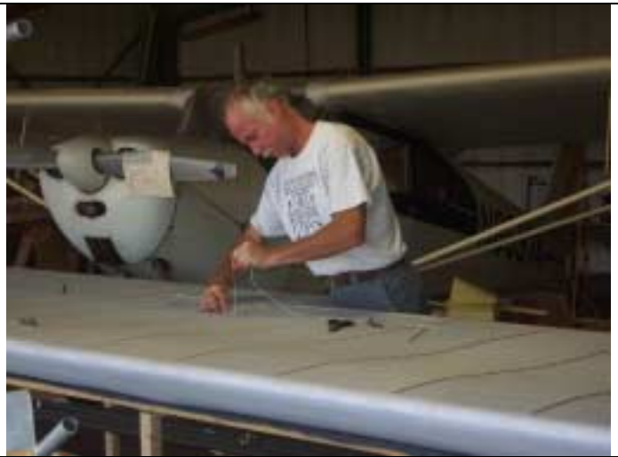
Gene Hubbard rib stitches a Pietyenpol wing
