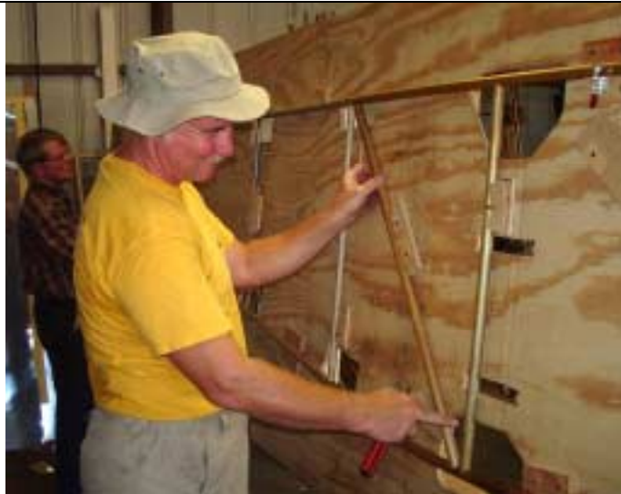
Gene Hubbard and Richard Kalling fit tubes to the Nieuport fuselage jig.
