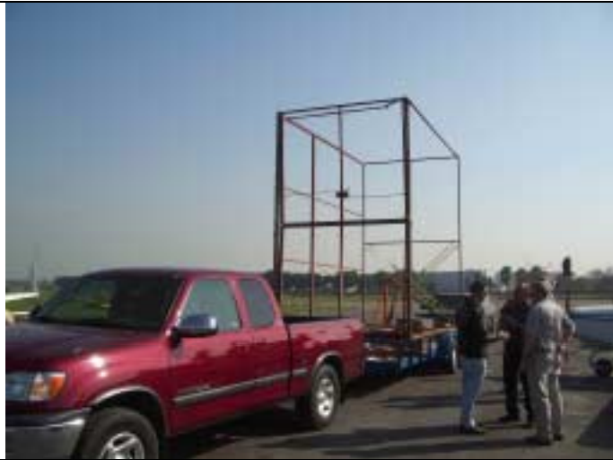
Hangar frame arrives at Brown despite bridge clearance 15' 1", hangar height, 15' 1 ¼"
