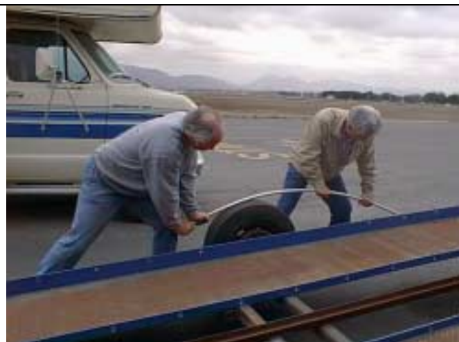
Gene and Joe bend a longeron tube per Nieuport plans
