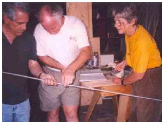
Joe and Gene cut tubing for Nieuport rudders.
