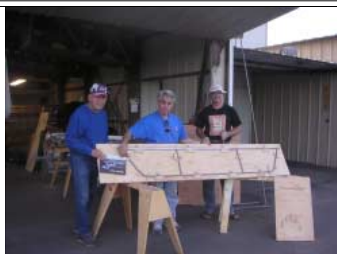
John Watts, Joe Russo and Gene Hubbard display a jiggged Nieuport stabilizer.
